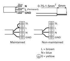
Step 6: Integrated downlight switch on/off.
